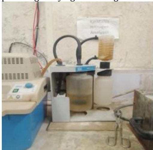
Figure : kjeldhal apparatus used in proximate analysis used to measure protein content
