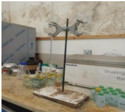
Figure Titration apparatus used in the last step of protein analysis after digestion
