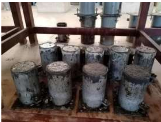
Fig. 3 (a) Casted samples immediately after moulding. (b) Samples prepared and ready for the curing process.
