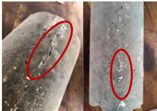
Fig. 5 Cracks filled through the precipitation of calcium carbonate.
