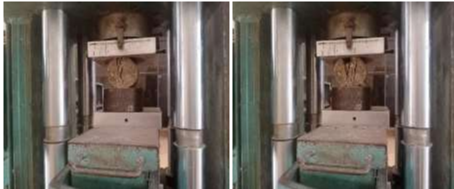
Fig. 4 Split tensile strength of cylinders in laboratory with UTM
