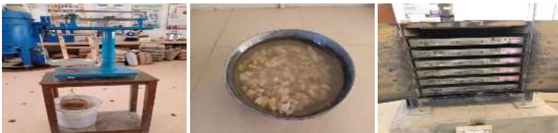
Fig. 1 (a) Specific Gravity Test (b) Water Absorption Test (c) Fineness Modulus Test of coarse and fine aggregate
