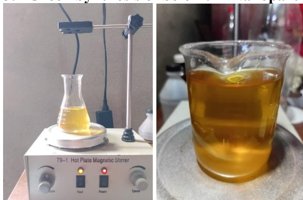
Figure 1: Synthetic setup for SeNPs using Binary extract of Moringa oleifera and Solanum lycopersicum
