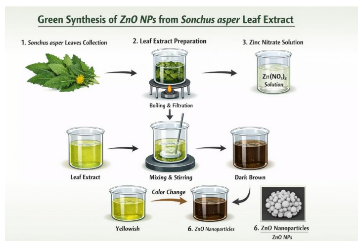
Figure 1: Showing Layout for the Synthesis of ZnO Nanoparticles
