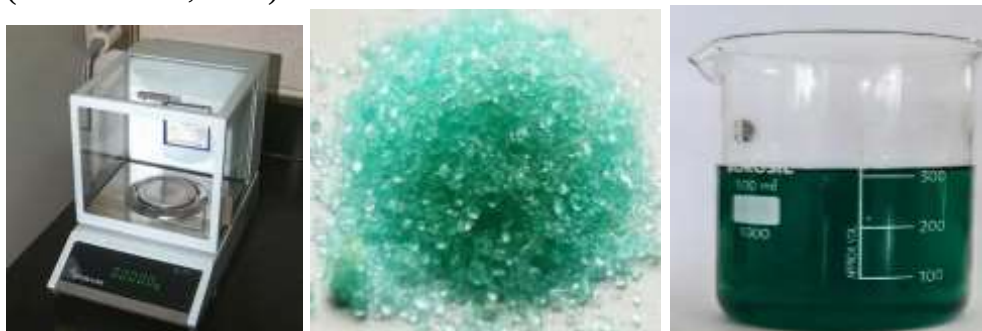
Figure 2: Preparation of 20mM NiSO 4 salt solution
