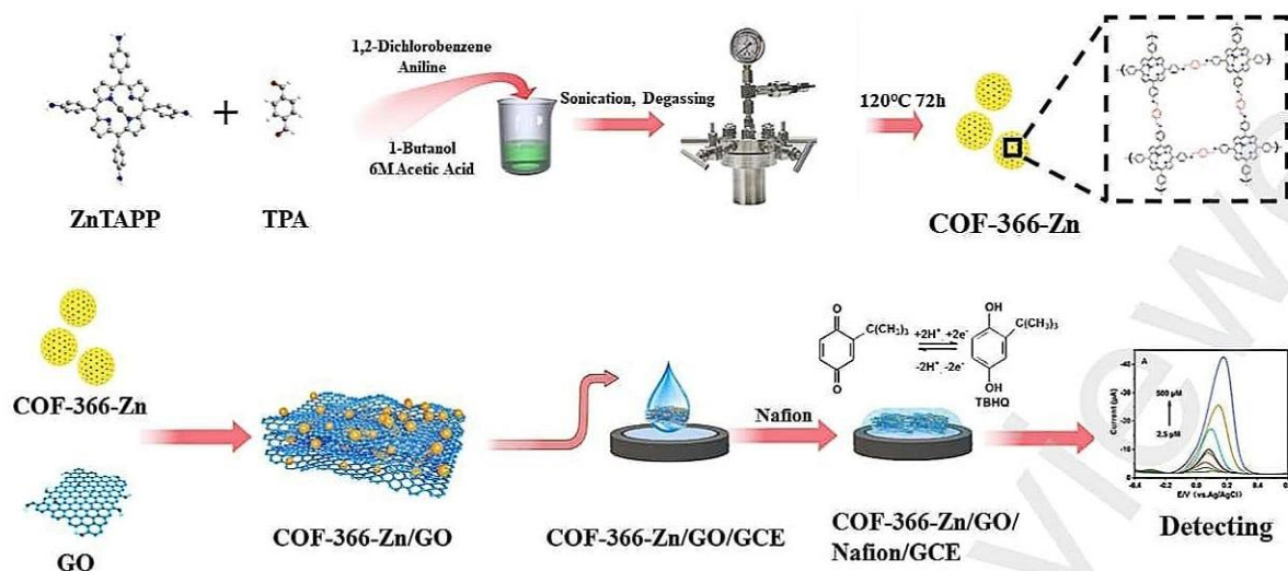
Figure 2.50 Synthetic Scheme of COF-366-Zn, COF-366-Zn/GO/Nafion/GCE, COF-366-Zn/GO/GCE and COF-366-Zn/GO (Metal-Porphyrin-based COF)
