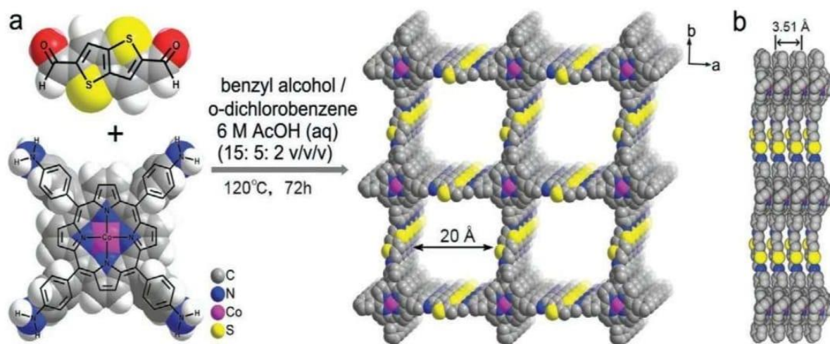
Figure 2.70 Synthetic Scheme of TT-Por(Co)-COF (Porphyrin-based COF)
