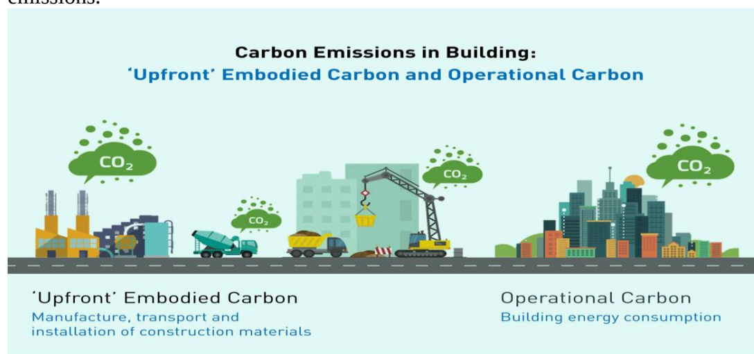
Figure No: 4 Conceptual framework of embodied carbon emissions within the infrastructure life cycle.
