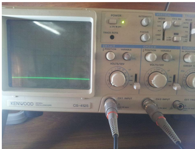
FIG 19 SCALE VOLTS/DIV ON OSCILLOSCOPE USING CHANNEL 2
